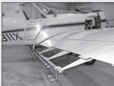
The nozzles that deflect the spray.
